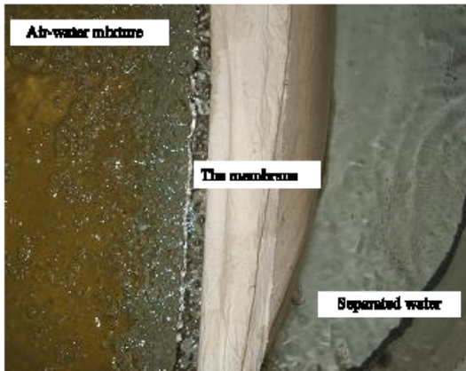
Fig. 4: Membrane which was used to separate water from bubbles
