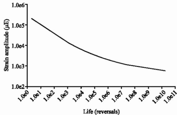
Fig. 4: The theoretical strain-life curve for the SAE 1045 steel
