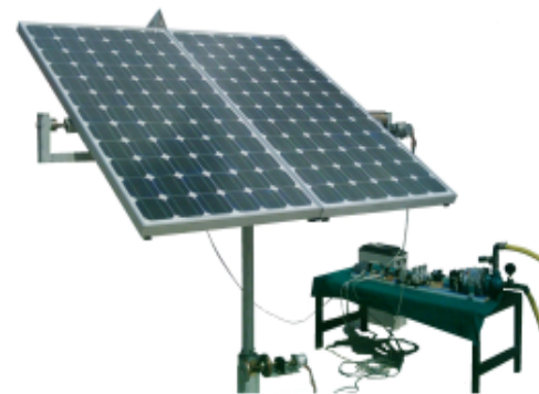
Fig 2: General view of solar monitoring pump system
