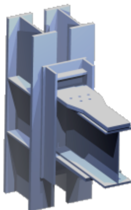
Fig. 2: 3D view of the proposed connection
