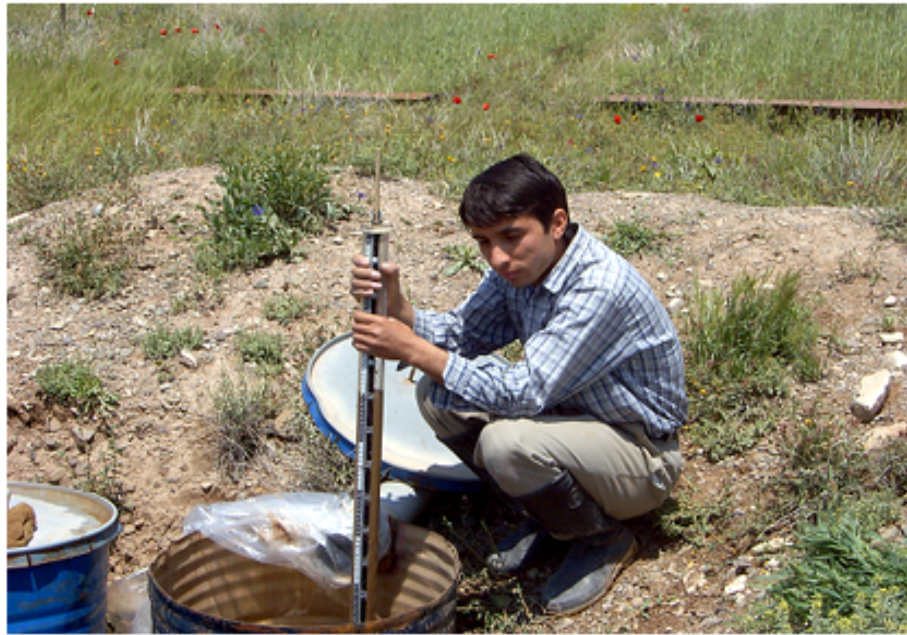
Fig. 1: Runoff and sediment sampling from collecting tank
