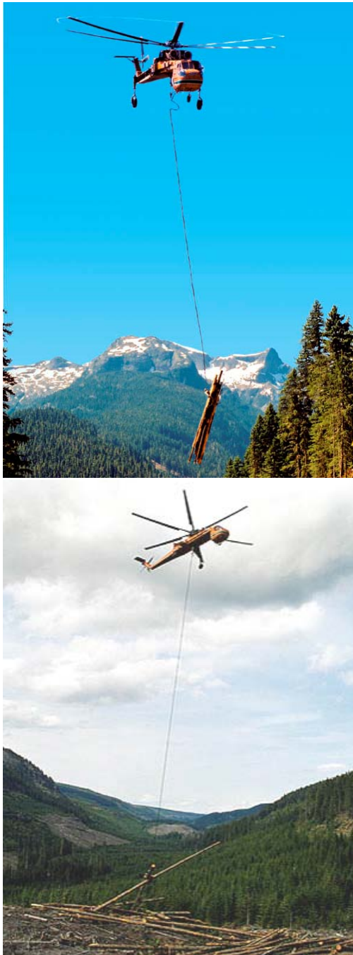
Fig. 1: Lifting (left) and landing (right) operations in helilogging (Ericson Air-Crane Inc., USA)
