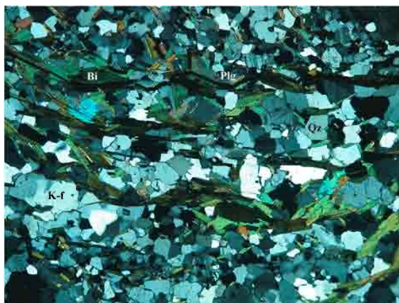
Fig. 4: Photomicrograph of a biotite granite from Malayer granitoid complex Western Iran, (Bt = Biotite; K-f = K-Feldspar; Plg = Plagioclase; Qtz = quartz)
