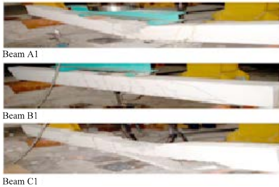
Fig. 7: Failure mode of tested specimens
