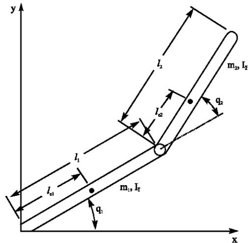
Fig. 1: Two link elbow robot manipulator
