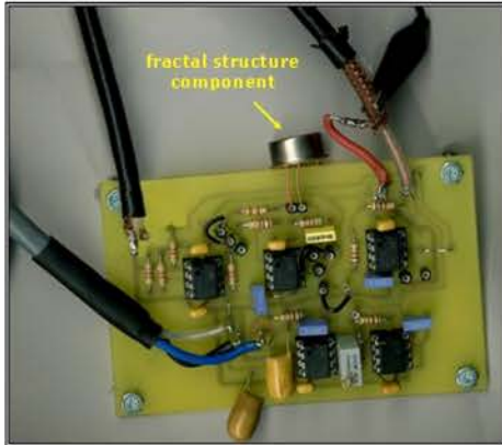
Fig. 11: Fractional PI controller circuit design
