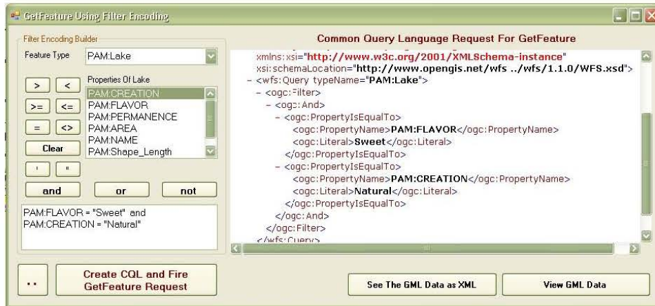
Fig. 6: User interface for introducing CQL statements and retrieve GML data from WFS server
