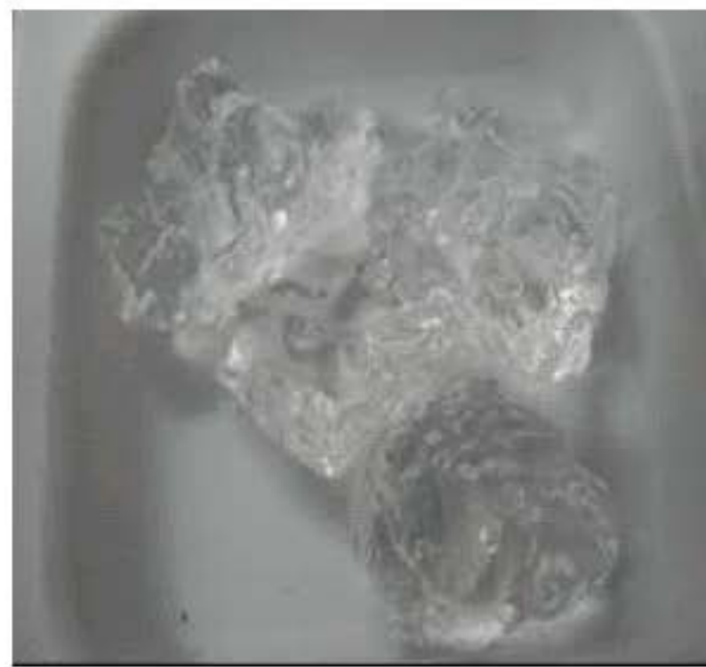
Fig. 4: Methanol soaked in aqua gel
