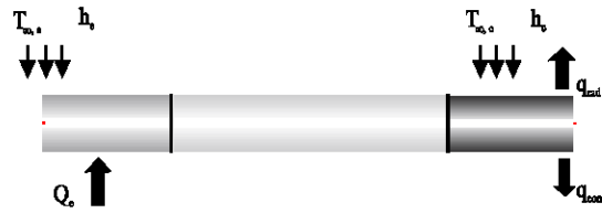
Fig. 2: Control volume for lumped capacitance analysis
