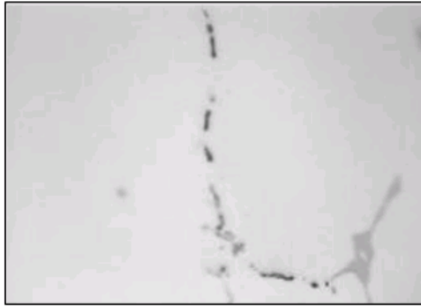
Fig. 4: Composition of continues M_{23}C_6 carbides on grain boundary, x500
