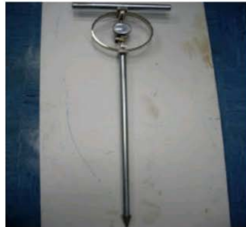
Fig. 2: Hand operated proving ring cone penetrometer
