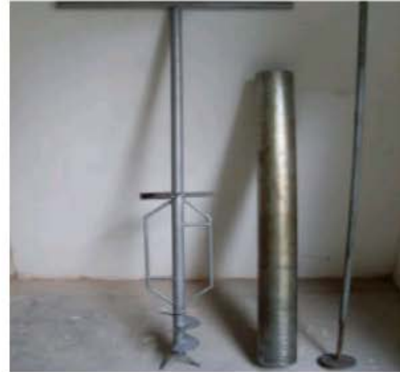
Fig. 3: Mixing tools for field column installation
