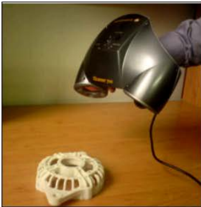
Fig. 6: Digitization of RP model by handheld laser scanner
