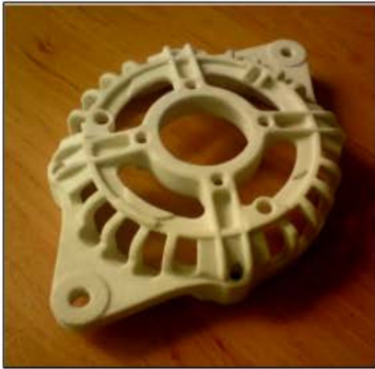
Fig. 3: The produced model of test part by 3D printing process
