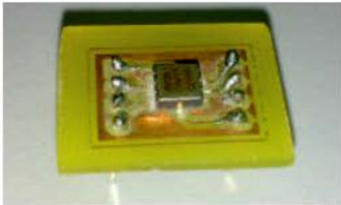
Fig. 4: Complete PCB for ADXL202E
