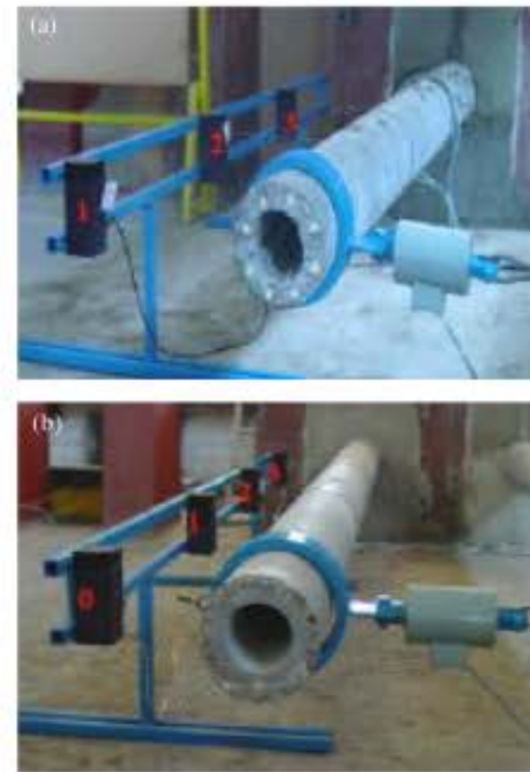
Fig. 5: Instrumentation of the test samples with LVDTs (a) the 3 m long column and (b) the 4 m long column
