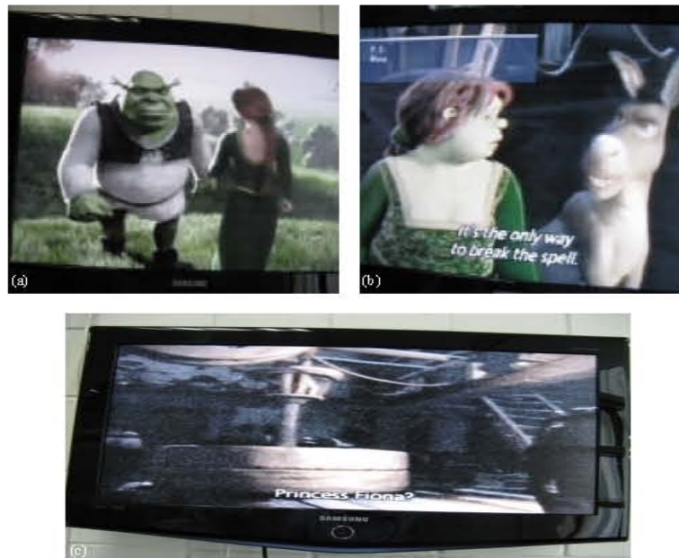
Fig. 9: Comparison of brightness for 1550 nm video signals; (a) original signal (before modulate) (b) 90% tapped signals (receive from ONU) and (c) 10% tapped signals (receive from PIM device)
