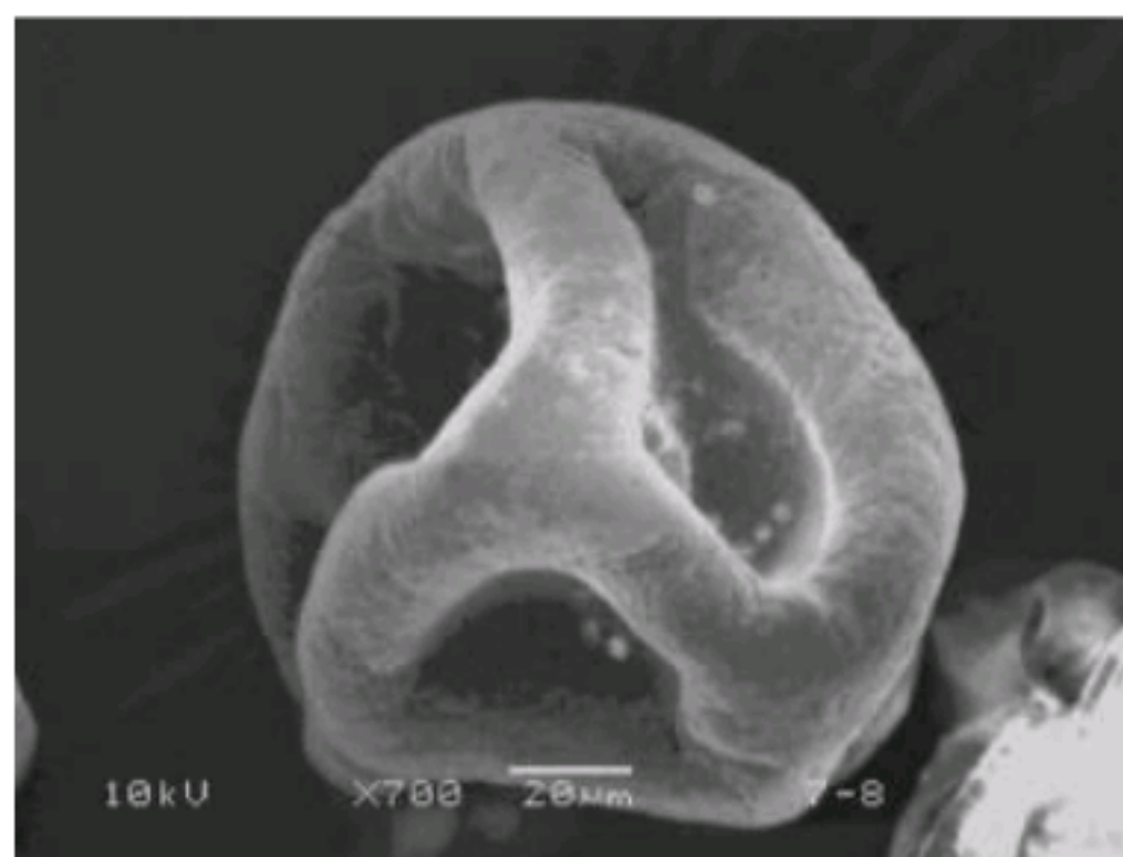
Fig. 6: Expanded SEM micrograph of methanol treated SF microparticles, bar scale = 20 μm
