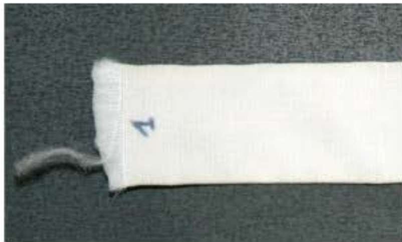
Fig. 2: Sample of tubular plain woven structure
