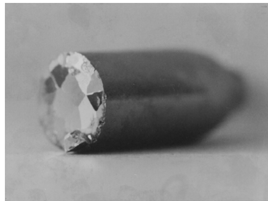
Fig. 5: Cross section of polycrystalline ingot
