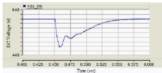
Fig. 15: DC link voltage
