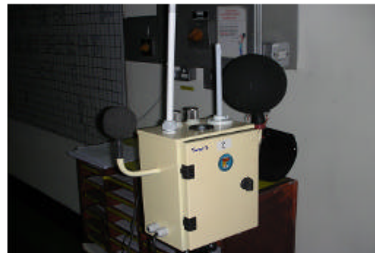
Fig. 1: Thermal Comfort Measurement (TCM) equipment
