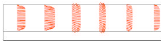
Fig. 6: Fluid flows at the entrance of single microchannel ( 0.001 \text{ m sec}^{-1} )
