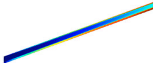
Fig. 8: Temperature distribution of single microchannel (200 kPa)
