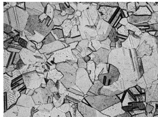
Fig. 1: Microstructure of the workpiece material nickel based alloy 242 (HI, 2009)
