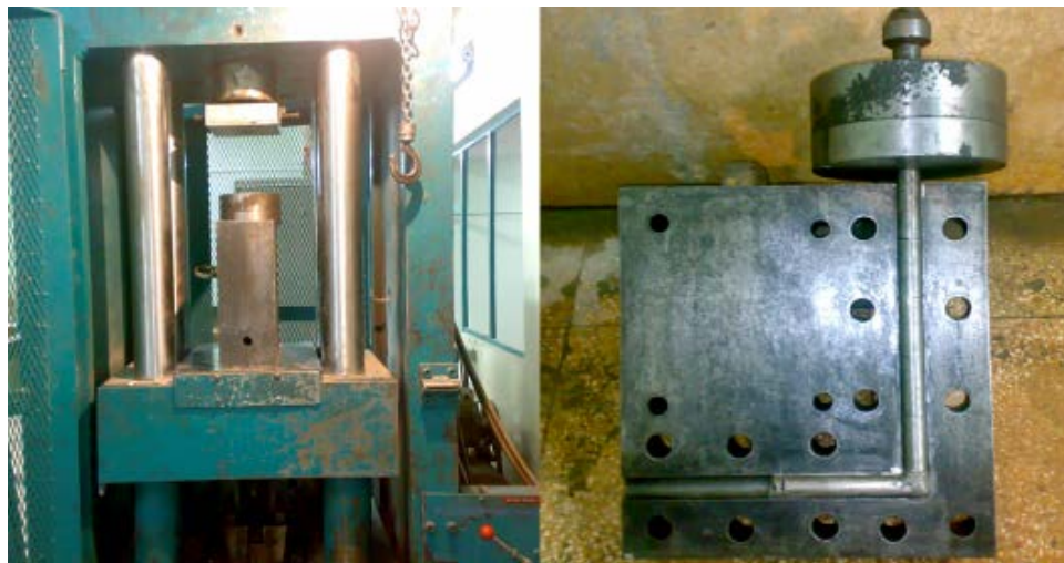
Fig. 6: The ECAP set-up for experimental work: hydraulic press and ECAP die set-up
