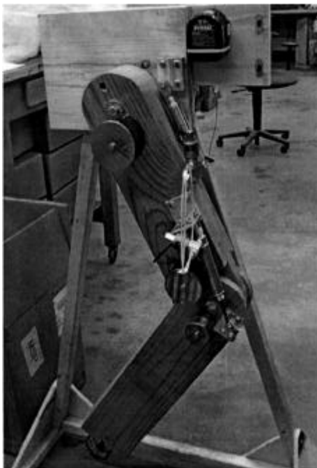
Fig. 4: Bench model physical prototype of energy storage orthosis (Durfee and Rivard, 2005)
