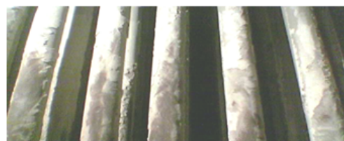
Fig. 2: Slag formed on the tubes
