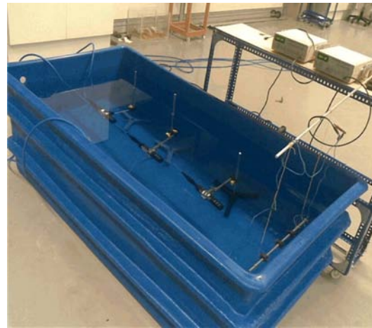
Fig. 2: Experimental set up of EM transmitter with three sensors
