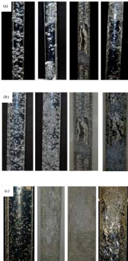
Fig. 4: Flow pattern inside (a) 21 mm; (b) 47 mm and (c) 95 mm, ID pipe vertical upward flow
