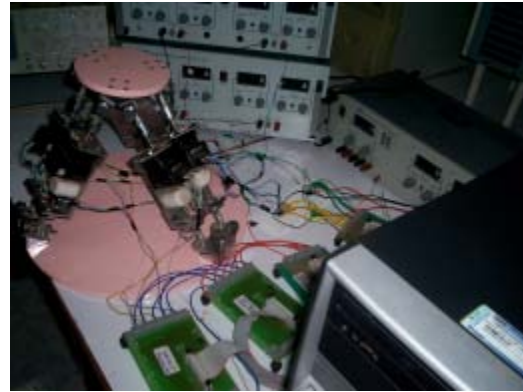
Fig. 9: Developed Stewart platform (PeilPOD 3-3)
