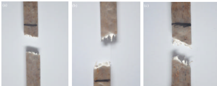
Fig. 3: Typical fracture specimens processed (a) at 70 bar pressure, (b) at 170°C and (c) at 190°C
