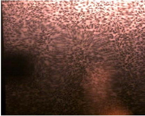
Fig. 3: The BOS image taken through gas flame media
