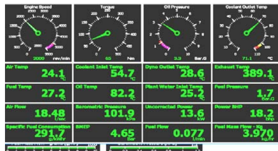
Fig. 3: Typical display of the engine test bed panel
