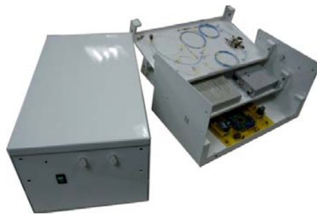
Fig. 3: MADS prototype developed to detect failure which occurs in the active FTTH's line
