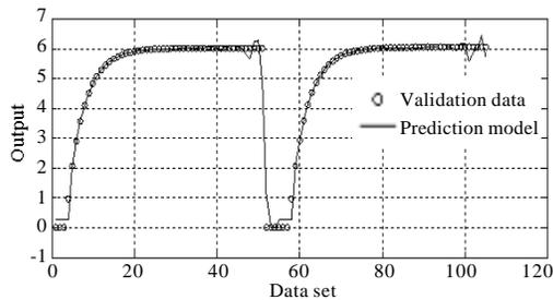
Fig. 4: Neural network validation performance for top end point composition (y1) with manipulation of top draw flow rate (u1) in perfect case
