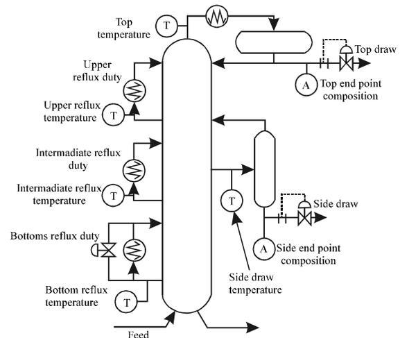
Fig. 2: Schematic diagram of “Shell” heavy oil fractionator (Maciejowski, 2002)
