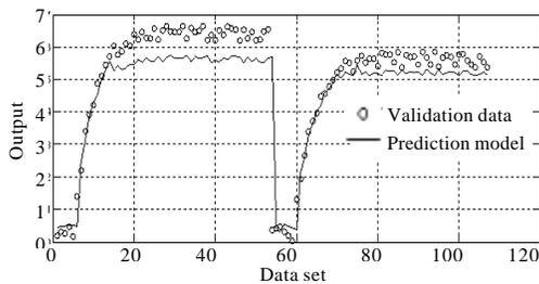
Fig. 6: Neural network validation performance for top end point composition (y1) with manipulation of top draw flow rate (u1) and measurement noise of 0.5
