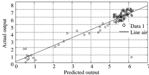
Fig. 8: Proportionality between actual and predicted validation data for top end point composition (y1) with manipulation of top draw flow rate (u1) and measurement noise of 1.0
