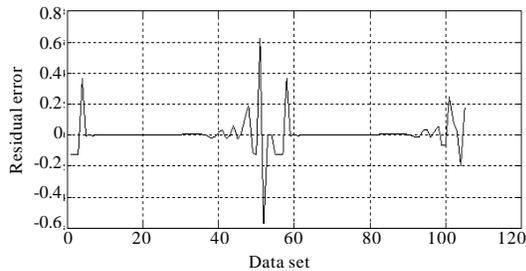
Fig. 5: Residual between actual and predicted validation data for top end point composition (y1) with manipulation of top draw flow rate (u1) in perfect case
