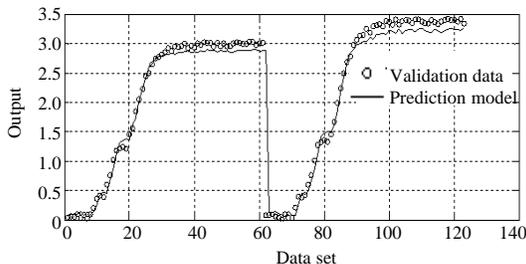
Fig. 10: Neural network validation performance for top end point composition (y1) in multiple input system with varied step time
