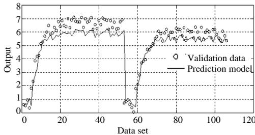
Fig. 7: Neural network validation performance for top end point composition (y1) with manipulation of top draw flow rate (u1) and measurement noise of 1.0
