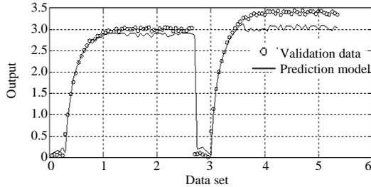
Fig. 9: Neural network validation performance for top end point composition (y1) in multiple input system with constant step time
