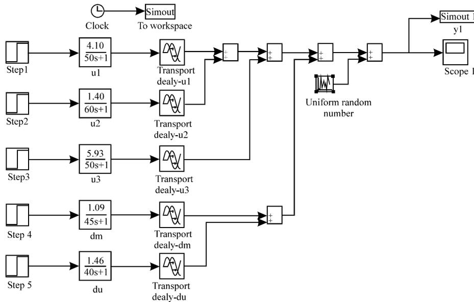
Fig. 3: Block diagram for combination of FOPTD system for real case simulation on generating top end point composition (y1) with the manipulation of top draw flow rate (u1)
