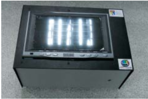
Fig. 3: The developed CATV tester unit
