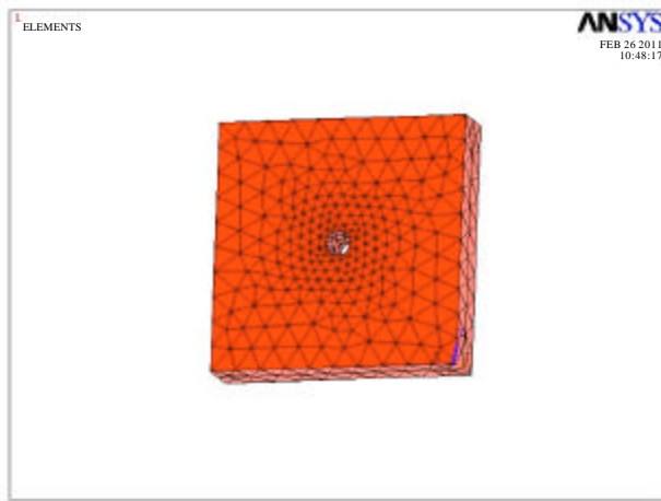
Fig. 16: Meshing of the injection model
