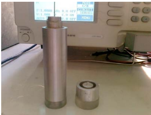
Fig. 1: A photograph picture of the big and small contact cylindrical capacitive sensors
