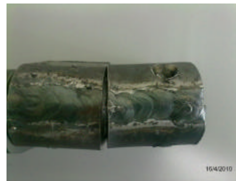
Fig. 4: The 3 mm crack in the specimen welded without vibration
