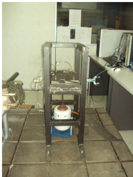
Fig. 1: The plate holder and the shaker for the experimental
