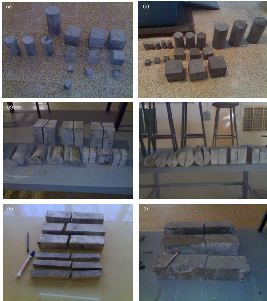
Fig. 1: (a-f) Samples of tested mortar having different specimen's sizes
