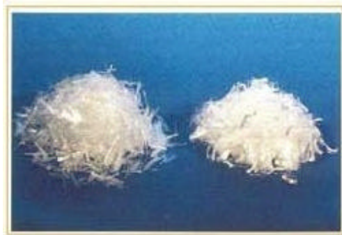
Fig. 3: Polypropylene fiber used in this study
