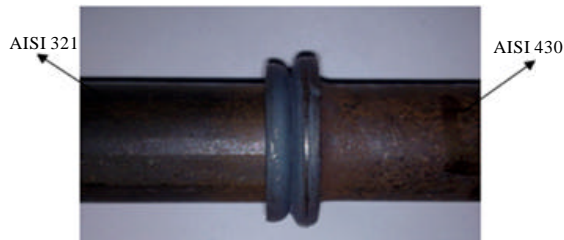
Fig. 4: Friction welded of AISI 321 and AISI 430
