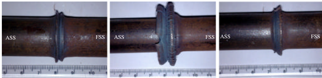
Fig. 6: Visual view of friction welded with various flash heights
