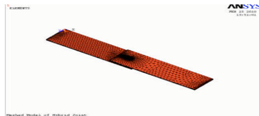
Fig. 3: Meshed model of hybrid joint
