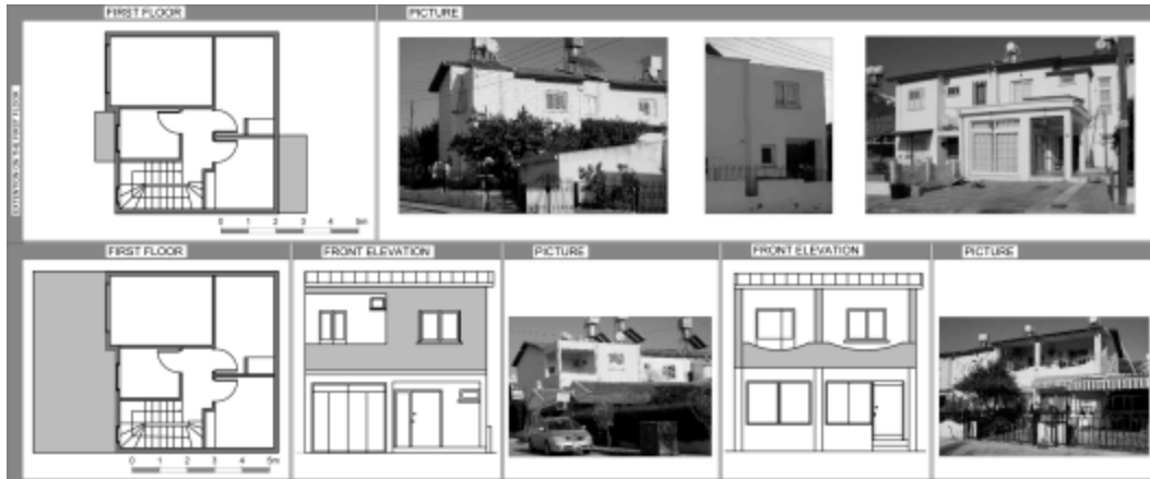
Fig. 5: Samples of extensions on the first floor of the social housing in Sakarya district
