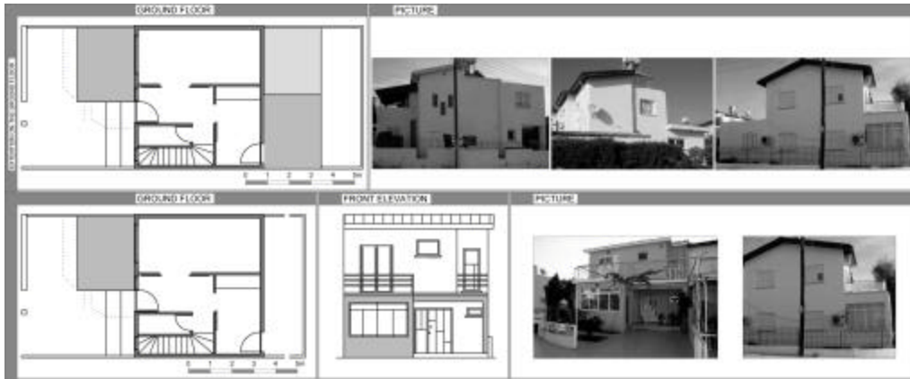
Fig. 4(a-f): Samples of extensions on the ground floor of the social housing in Sakarya district
