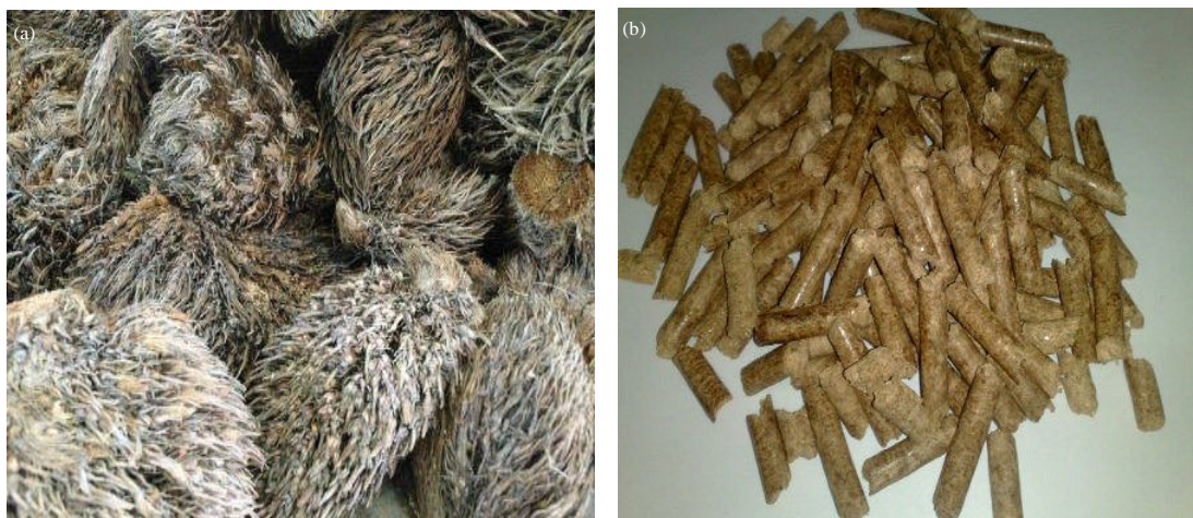
Fig. 1(a-b): (a) Empty fruit bunch (EFB) and (b) Empty fruit bunch (EFB) briquette
