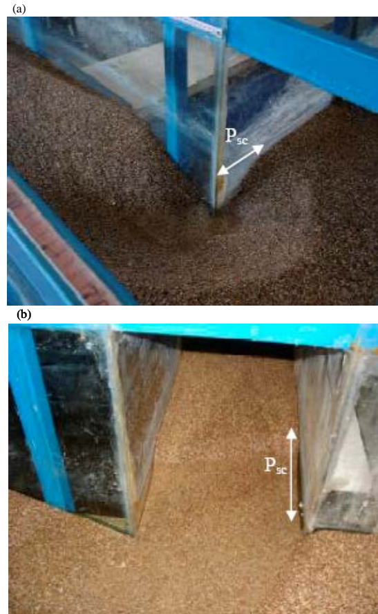
Fig. 2(a-b): Penetration of scour hole into tributary channel. (a): Scour hole reaches the toe of the lateral channel wall closer to the downstream junction corner and (b): Scour hole reaches both lateral channel walls
