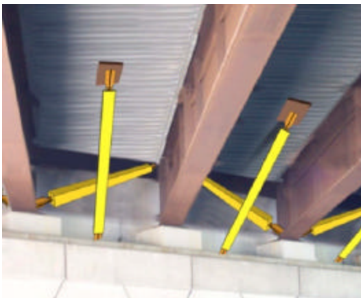
Fig.10:New detail of ductile end diaphragm by using Buckling Restrain Braces (BRBs) (Celik and Bruneau, 2009)
