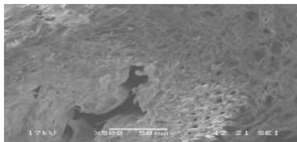
Fig. 3: Scanning electron micrograph showing single strand of coir fibre (x250)
